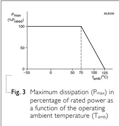
**Fig. 3** Maximum dissipation (P<sub>max</sub>) in percentage of rated power as a function of the operating ambient temperature (T<sub>amb</sub>)
